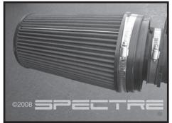
Step 15 Carefully insert the air filter over MAF sensor assembly and secure with the provided hose clamps.
