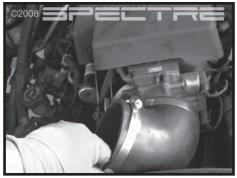
Step 10 Slide the 4" angled coupler and two 4" hose clamps over the throttle body. Do not tighten the clamps at this time.
